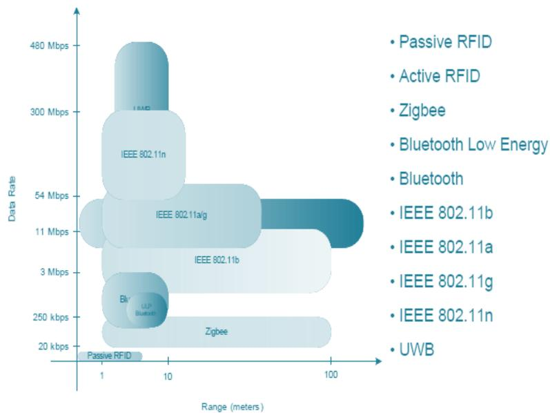
Figure 1. Potential wireless standards for medical applications source: Texas instruments
