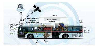
TI Jacinto 6-based solution, HD disassociated displays (for the BDC), Ethernet cameras, Dual band Wi-Fi, 4G connectivity and navigation system with world-wide coverage
